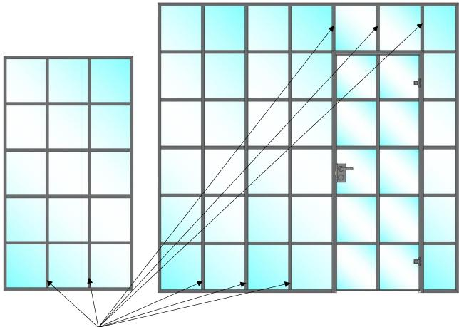
3-5. Measure the vertical bars and cut to both sides.Use an electric shortener saw with aluminum blade for best results.You will also need spirit level, tape measure, spray can and grout-gun
