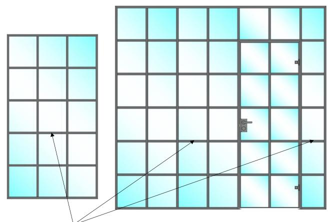
**3-6.** Then measure the horizontal bars and cut to both sides. Use an electric shortener saw with aluminum blade for best results. You will also need spirit level, tape measure, spray can and grout-gun
