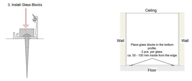
**1-6.** Mount the glass, make sure you have glass blocks mounted at the bottom. (For easier to move around on the glass, you can use a window lifter.)
