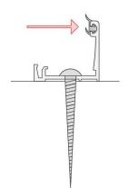
**1-5.** Install glass blocks at the bottom of the profile, 2 bricks for each glass. The blocks are ca. 50 - 100 mm from inside the corner.
