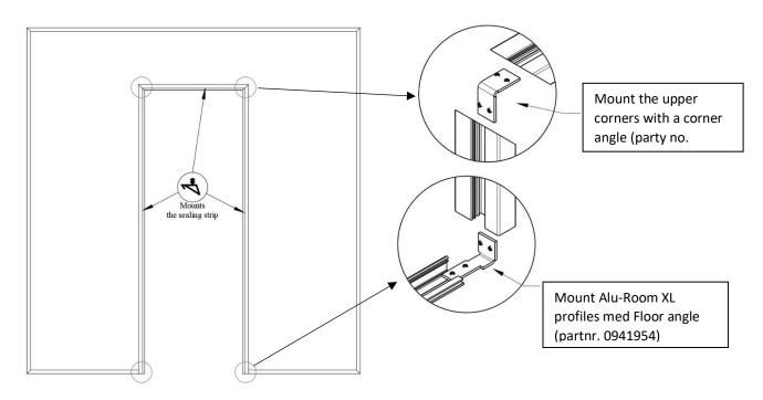
**1-9.** Scan the profiles, start with the top profile, cut it to the full width of the hole. 45 degree cut against wall, and <u>90 degree cut against door frame</u>.
